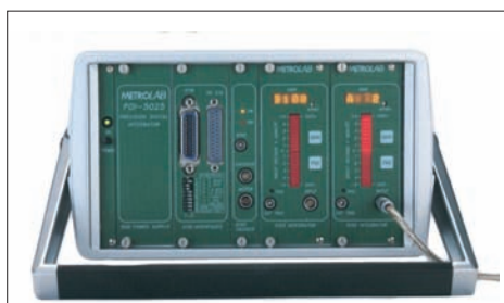
Figure 2. Metrolab's Precision Digital Integrator PDI5025, for decades the accepted standard for high-speed integrators, also based on a CERN design.
